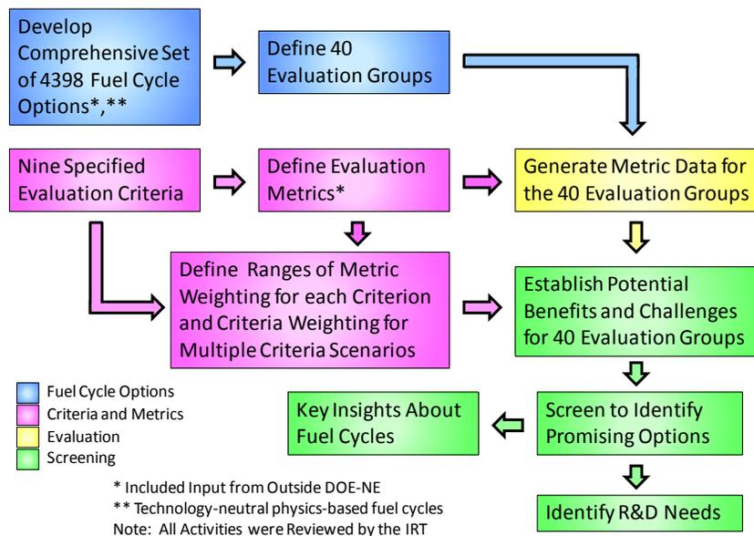
Figure 2. Nuclear Fuel Cycle Evaluation and Screening Process.
